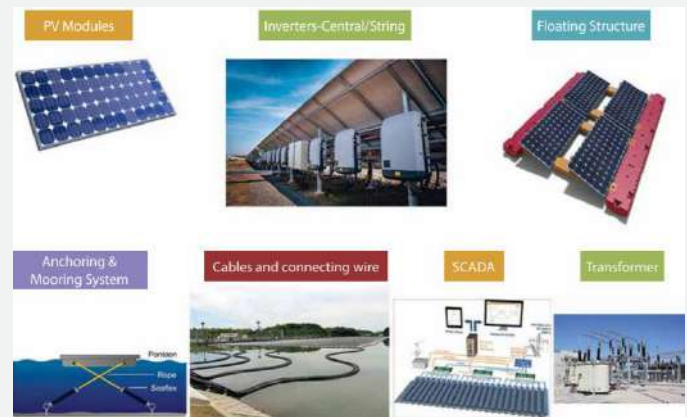
Figure 1. Major Components of FSPVs, Source: "Floating Solar Photovoltaic (FSPV): A Third Pillar to Solar PV Sector?", authored by Mohit Acharya and Sarvesh Devraj
