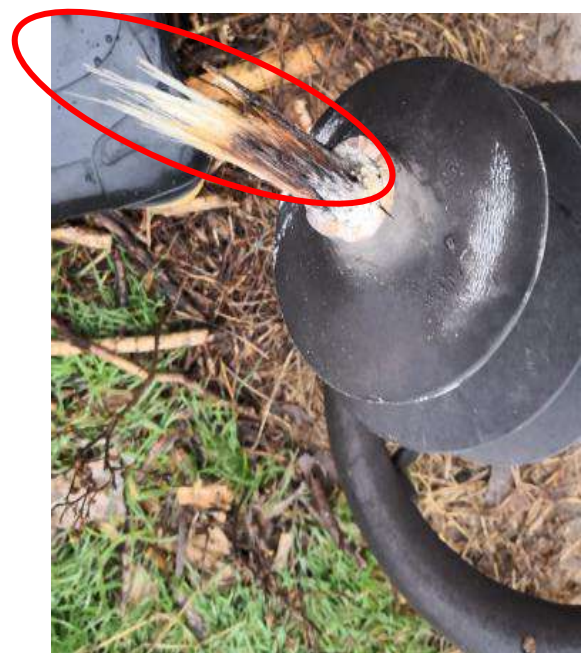
Figure 3 Fracture and mandrel at the fracture
