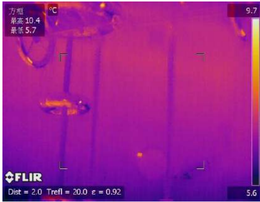
Figure 9 Insulator infrared temperature measurement test diagram
