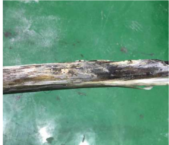
Figure 7 The mandrel appears pulverized and carbonized.
