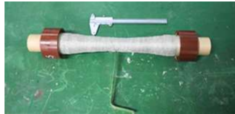
Figure 1. Test sample of insulating material PPLP insulation performance
