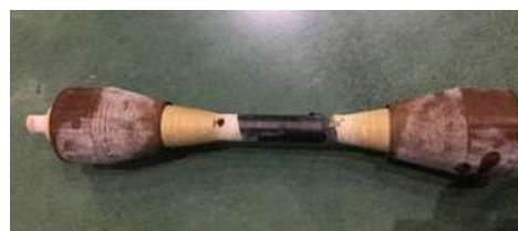
Figure 9. Breakdown diagram of power frequency withstand voltage test sample.
