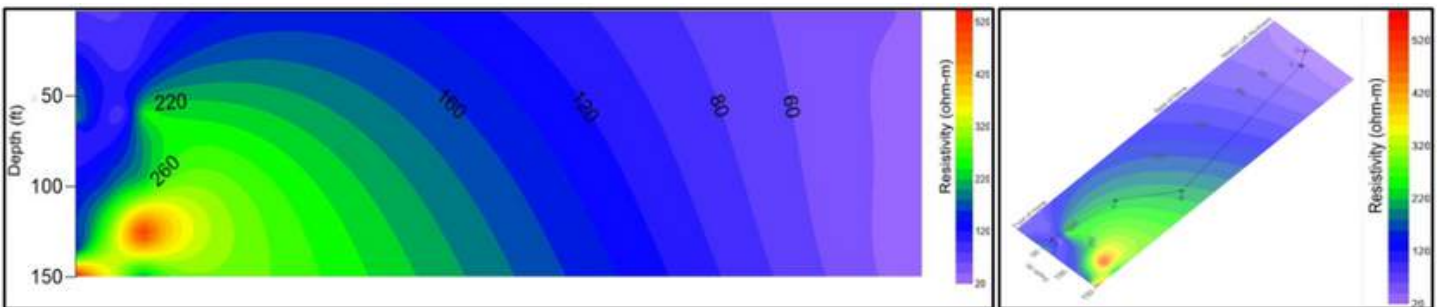
Figure 3: Main 2D Resistivity Profile of the Left abutment of Khanpur Dam
